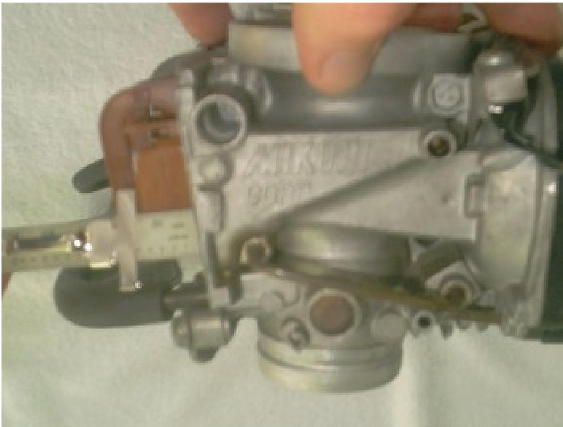
If you find that your floats are not within spec or you're experiencing a float height related problem, the height is altered by bending the metal tab. Go easy here. A little bit goes a long way. You don't have to remove the float assembly to alter the height, I just did that in this picture for the sake of clarity.
